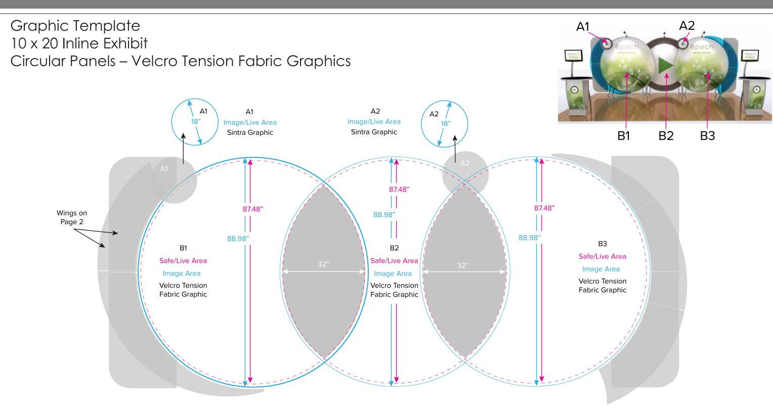
Velcro Tension Fabric Note: 1/2" Hook Velcro on Front Perimeter of Graphic
